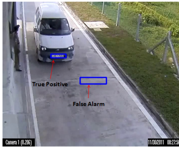
Fig. 3. Result of applying AdaBoost algorithm with Haar-like features in our dataset for license plate localization.
